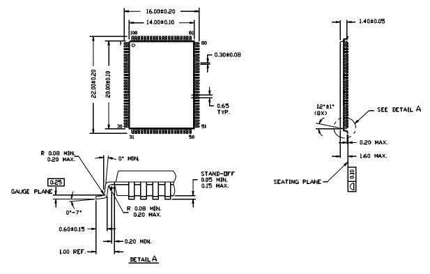
DIMENSIONS ARE IN MILLIMETERS.
